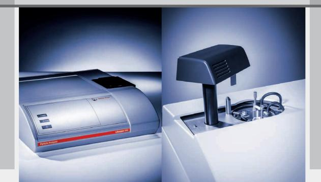
Integrated mechanical stirrer, peristaltic pump, and ultrasonic probe
