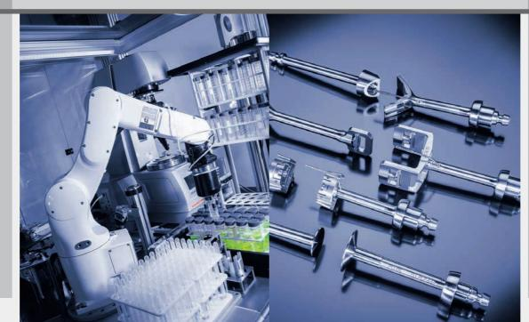
Measuring systems: Three-point-bending, dual cantilever, single cantilever, solid rectangular fixture, compression system
