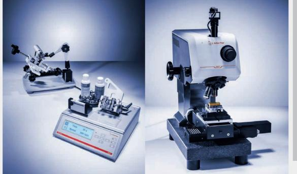
Friction force: Resolution: 100 µN Max. friction force: 200 N
