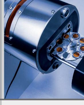
HPC 900: T: 25 °C to 900 °C, p<sub>max</sub>: 100 bar
